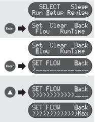
Press 🖸 to decrease the pump flow rate. Fewer arrow symbols are displayed on the LCD screen to indicate the reduced flow rate
