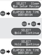
On the 'SELECT Hold' screen cycle to the 'Hold' option and press to stop the pump running and display the Hold menu screen, which also shows the current elapsed runtime.
